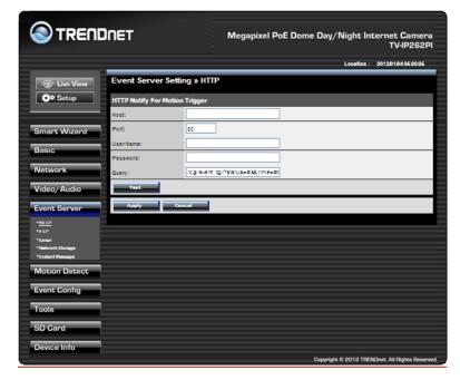
When you complete the required settings for HTTP Notify for Motion Trigger, FTP, Email, Network Storage, or Instant Message, click **Test** to test the related configuration is correct or not. Once the camera connects to the server successfully, click **Apply**.
